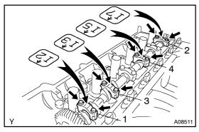
(2) Uniformly loosen and remove the 8 bearing cap bolts on the No.2, No.3, No.5 and No.7 bearing caps, in several passes, in the sequence shown.
