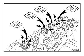
(3) Uniformly loosen and remove the 8 bearing cap bearing cap bolts on the No.2, No.4, No.5 and No.6 bearing caps, in several passes, in the sequence shown.
