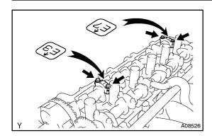
(5) Alternately and uniformly loosen and remove the 4 bearing cap bolts on the No.3 and No.7 bearing caps.
