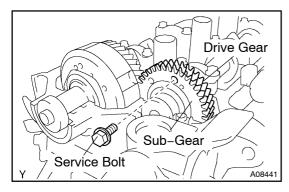
(2) Secure the intake camshaft sub-gear to the drive gear with a service bolt.
