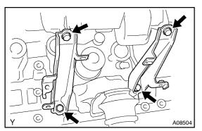
27. REMOVE NO.1 AND NO.2 AIR INTAKE CHAMBER STAYS
