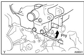
(b) Lift the cylinder head from the dowels on the cylinder block, and place the cylinder head on wooden blocks on a bench.
